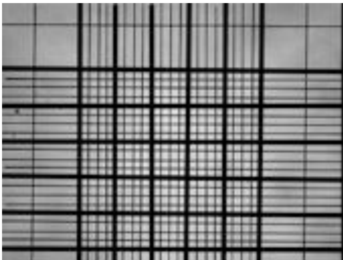
Figure 2b. Diagram of the central part of the grid (C). Note that the 0.04 mm 2 squares (A) are each divided into 16 smaller squares. At the upper left and right are two of the 0.0625 mm 2 corner squares (B).
